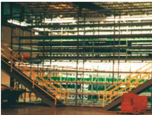
Multi-level Wide Span Pick Module
